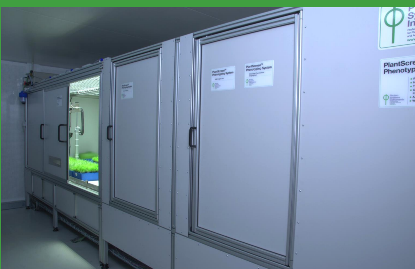
Automated phenotyping of up to 320 small- and mid-size scale plants in controlled environment in PlantScreen™ Compact System.
