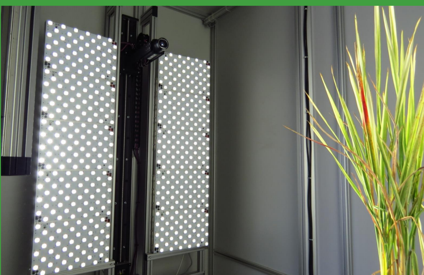
Automated phenotyping of 270 plants up to 1.5 in height in greenhouse environment in PlantScreen™ Modular System.
