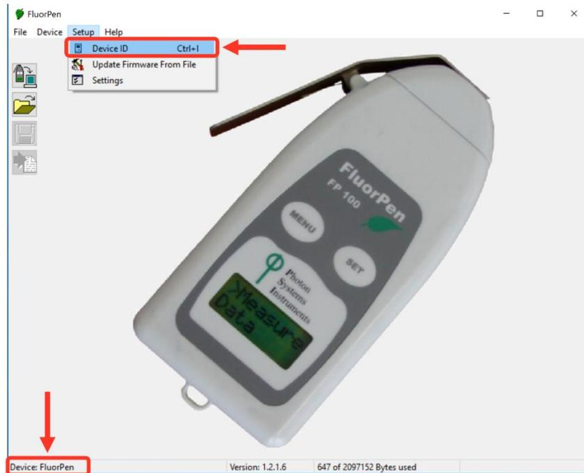
Fig. 20 Connecting FluorPen device with Software.
