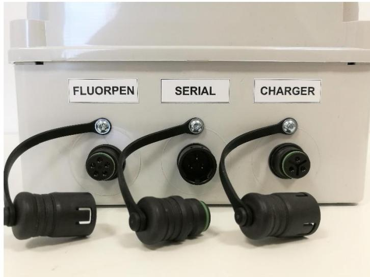
Fig. 33 Connectors of Standard Battery Pack.
