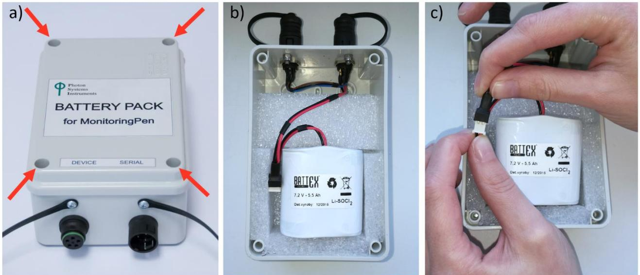
Fig. 36 Battery replacement for Extended Temperature Range Battery Pack.
