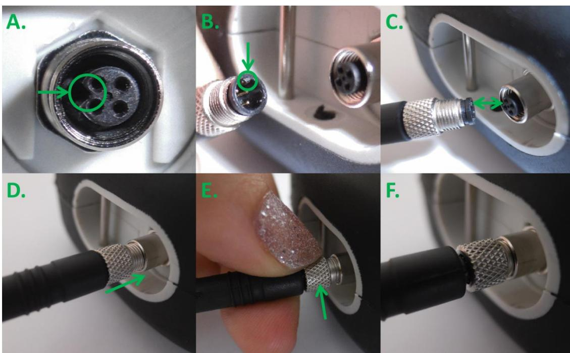
Fig. 12 How to connect FluorPen with USB cable.
