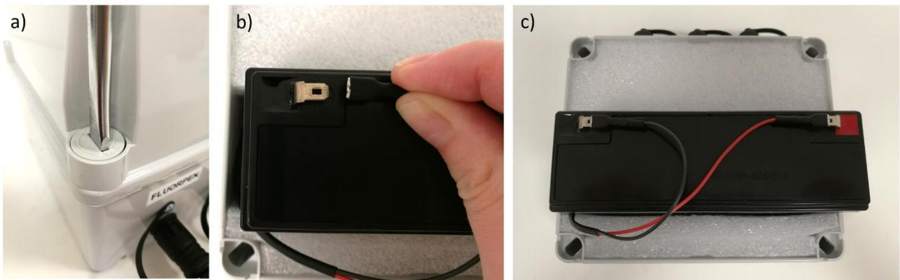
Fig. 34 Replacement of battery in a Standard Battery Pack.
