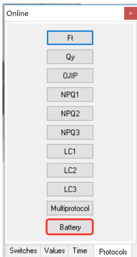
Fig. 37 Online control window enables checking of battery status.
