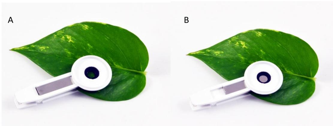
*Fig. 39 The detachable leaf clip in open (A) and closed (B) position.*
